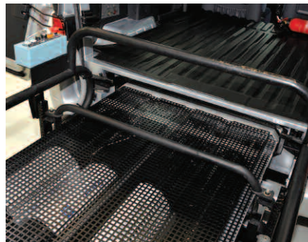
Removable hydrogen storage rack
